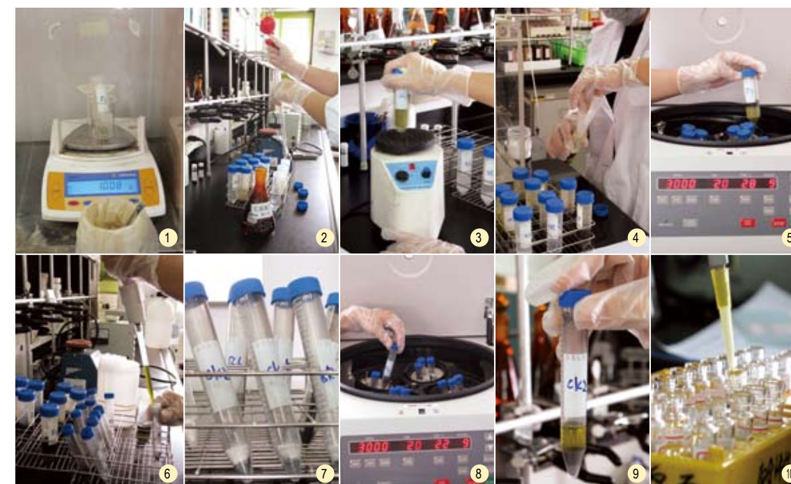
QuEChERS (Quick, Easy, Cheap, Effective, Rugged, and Safe) Multiresidue Method
